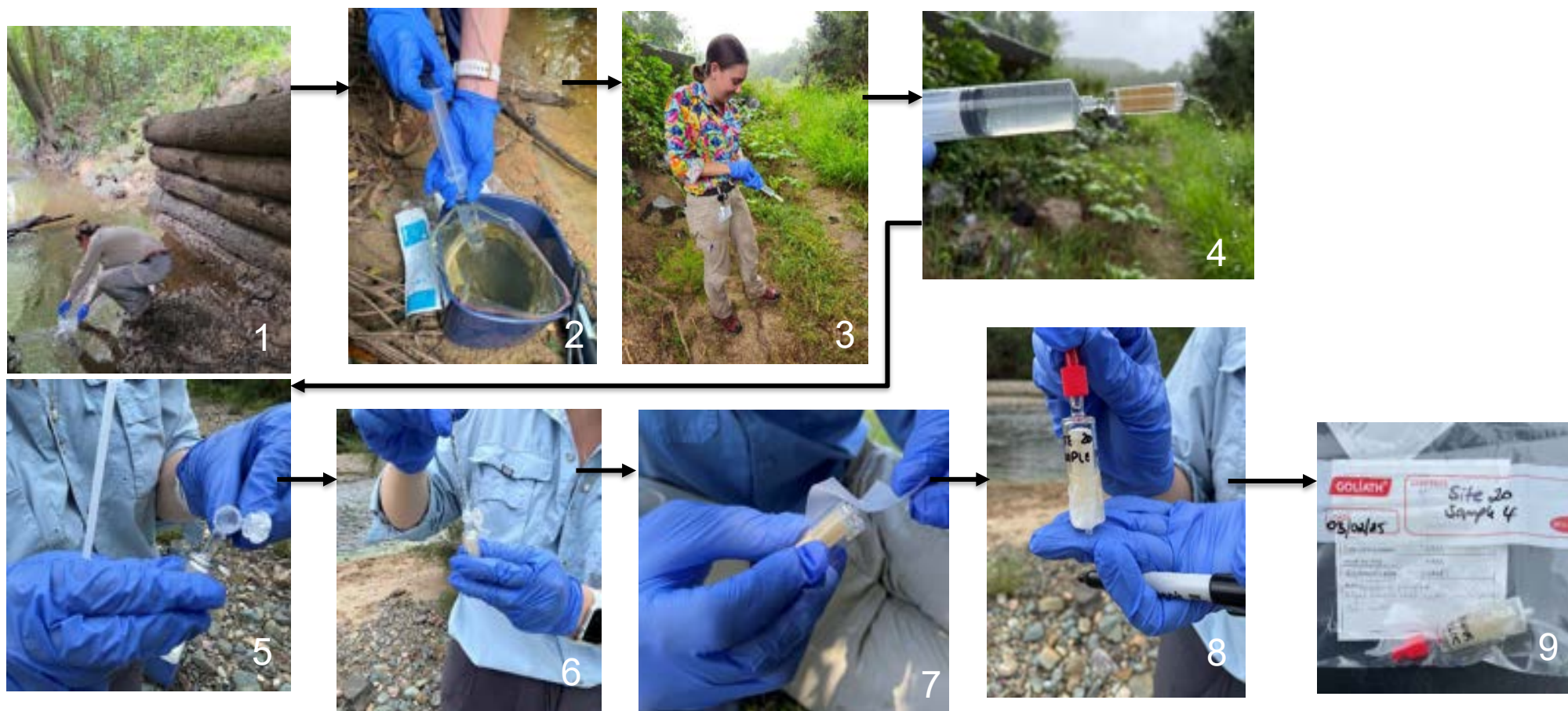
Image 17: eDNA sampling process: 1: water sampled collected, 2: water drawn into syringe, 3: water pushed through syringe, 4: water filter with genetic material, 5: preservative added to filter, 6: preservative saturated filter, 7: parafilm secured to seal the preservative, 8: sample labelled, 9: sample and site notes for the University
