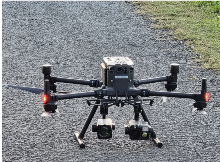
Image 1 The DJI Matrice 300 with H20N thermal/optical camera and GL60 Zoom spotlight was the primary drone and payload used to for the thermal drone survey.
