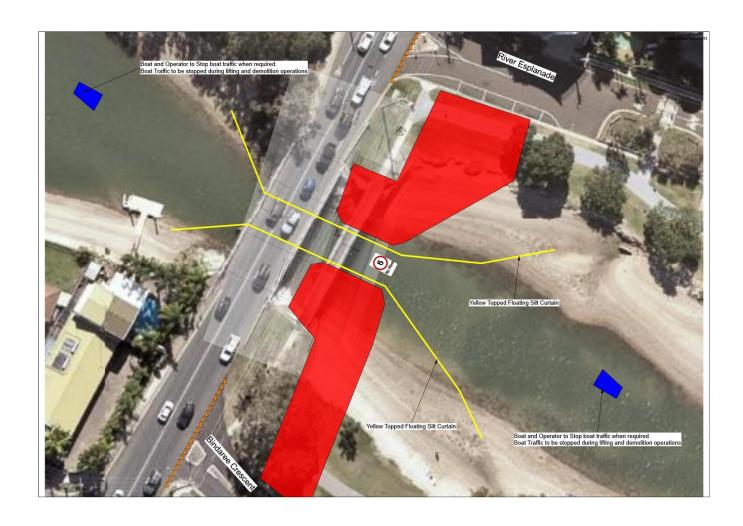
Figure 1. Location of temporary bridge piling platforms. Mayes Canal, Mooloolaba
