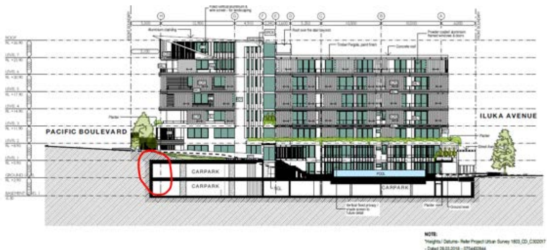
Figure 13: Location of basement wall to be constructed to the standard of a seawall
