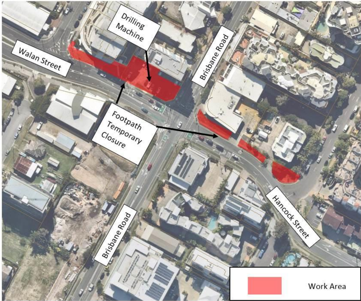
Figure 1. Site of gas main relocation works and temporary traffic arrangements in place as specified
