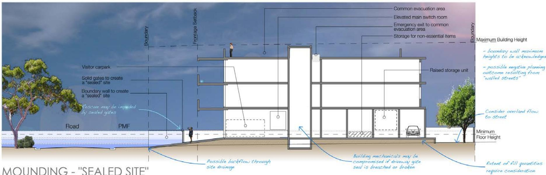
**Figure 10** Multi-Unit - Sealed site section
