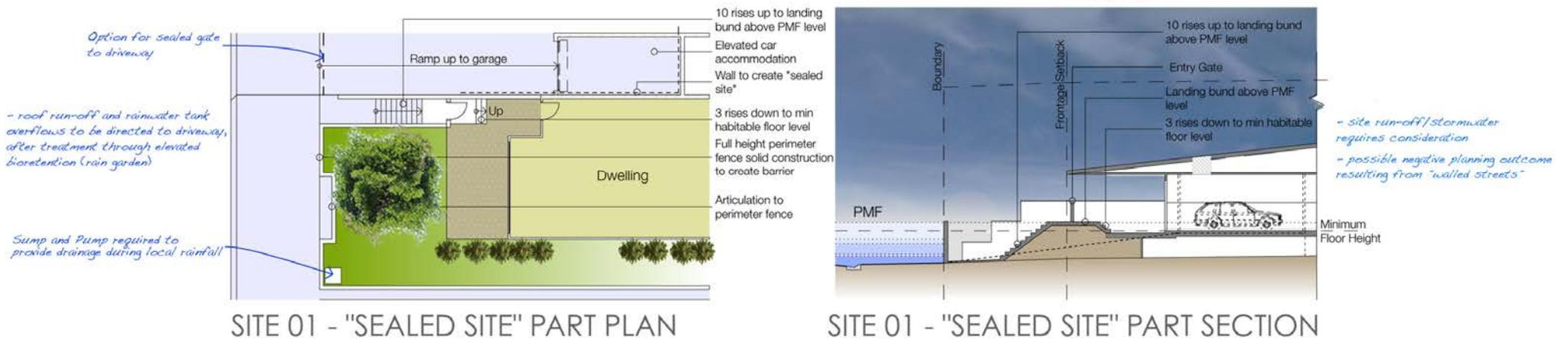
**Figure 7** Duplex - Sealed Site Sections
