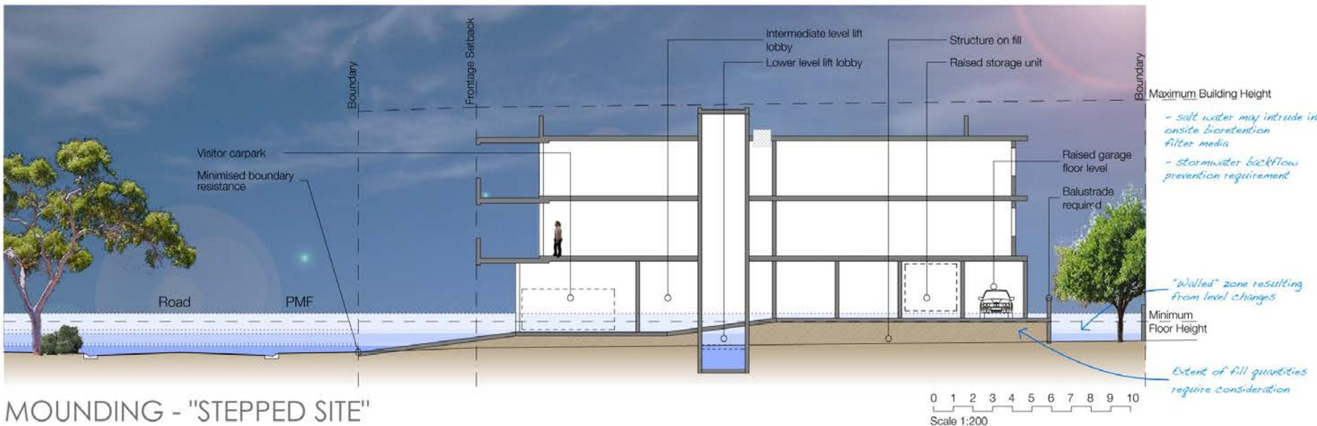
**Figure 11** Multi-Unit - Stepped site section
