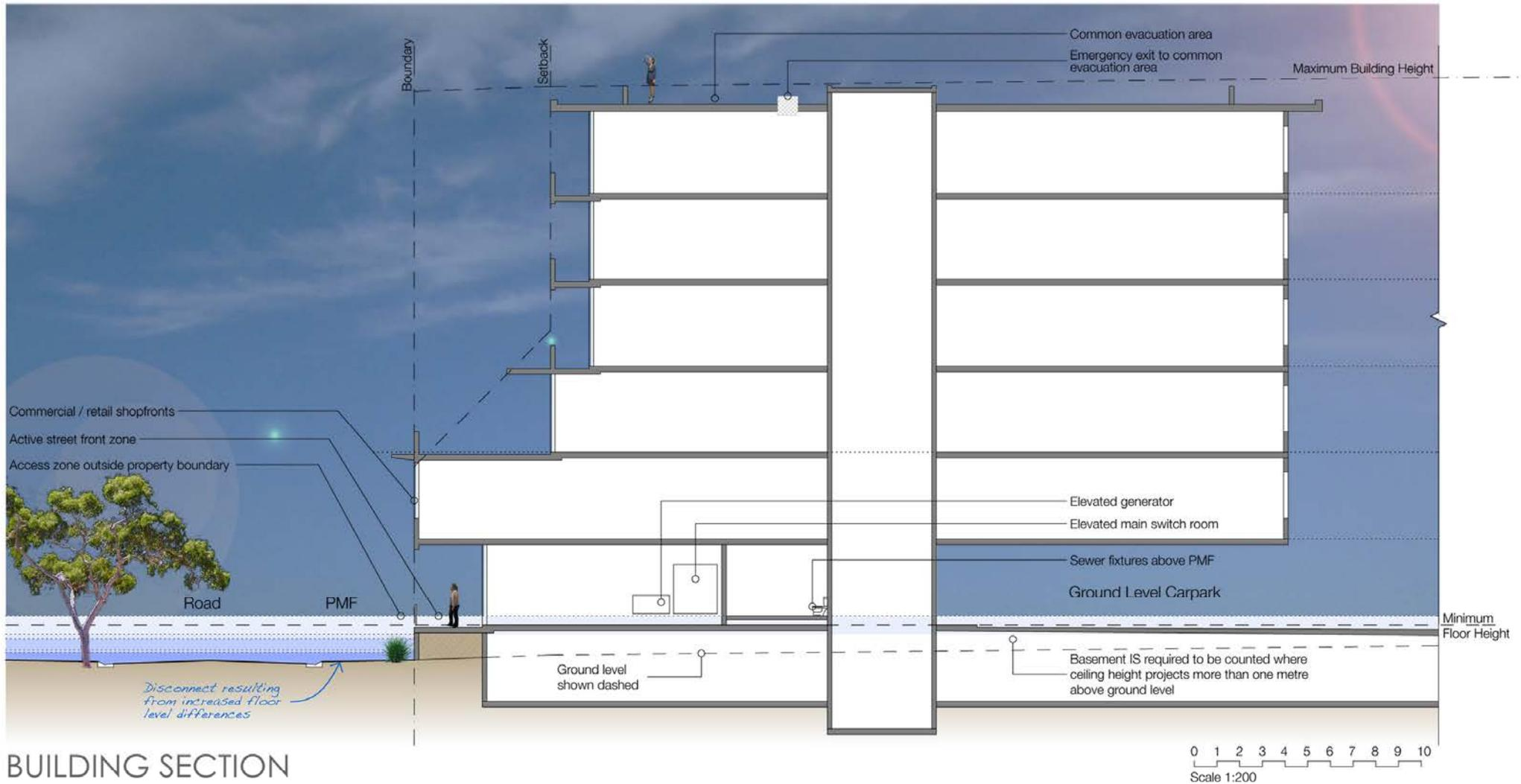
**Figure 18** Commercial - Building section
