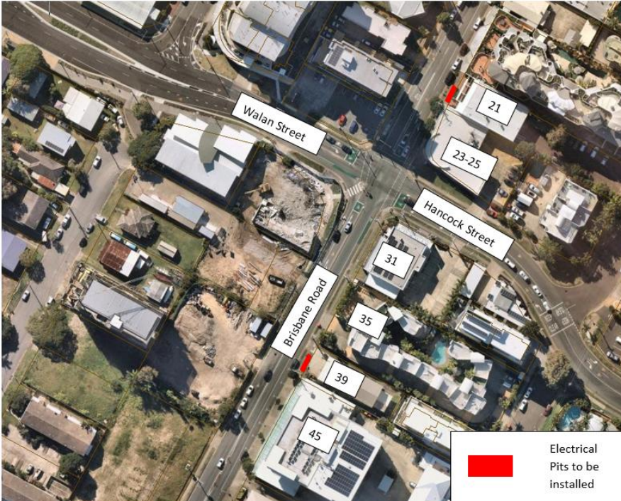
Figure 1 Location of Energex pit works adjacent to 39 Brisbane Road, Mooloolaba including construction area across driveway and to carports
