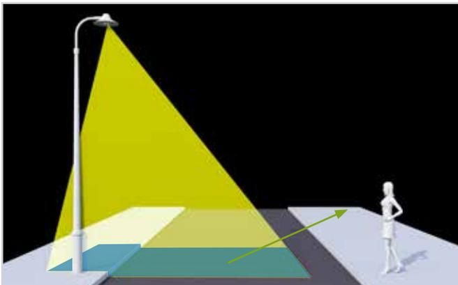
The luminaire emits light (yellow cone) resulting in light on the road (blue area; illuminance). The light is then reflected towards the eye of the viewer (green arrow; luminance).
