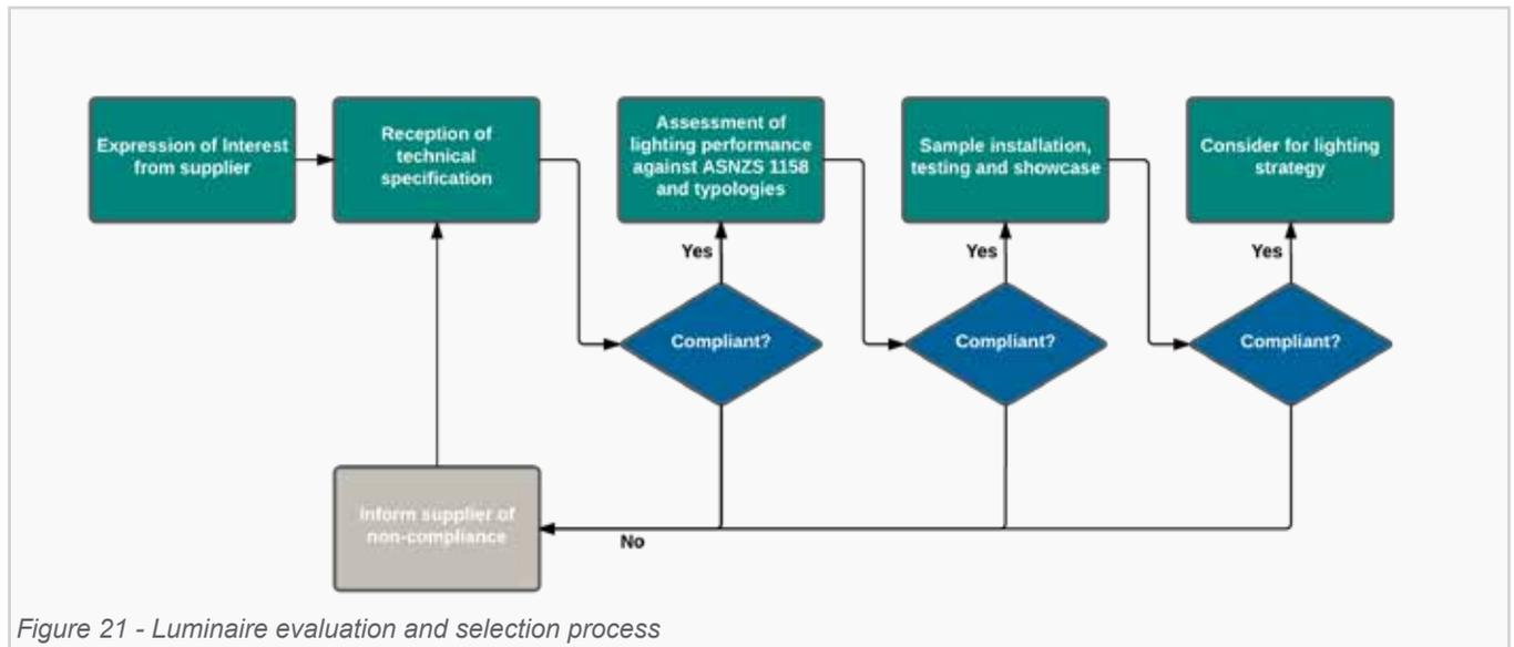
Figure 21 - Luminaire evaluation and selection process
