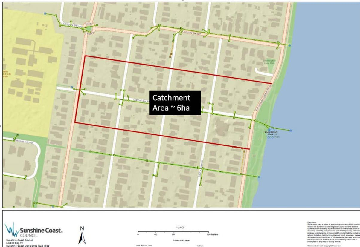
**Figure 4 – Catchment area treated by Earnshaw Street Vegetated Infiltration Basin**
