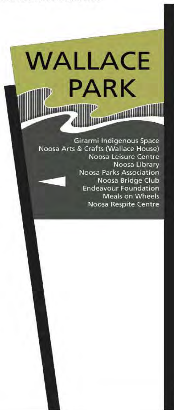
PRECINCT IDENTITY / ENTRY SIGNAGE WITH LIST OF FACILITIES EXAMPLE ONLY FOR DISCUSSION PAINTED METAL POSTS AND PANELS WITH BLACK AND WHITE LETTERING EXAMPLE HAS BEEN BASED ON IDENTITY SIGNAGE AT MOFFAT BEACH
