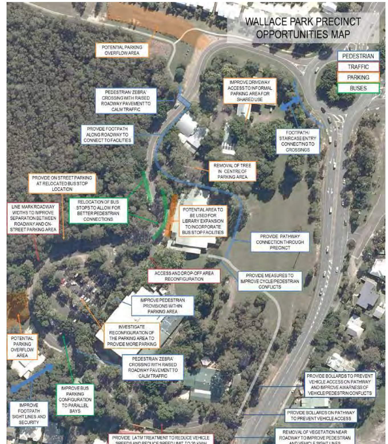
Diagram extracted from Wallace Park Precinct Master Plan: Traffic Impact Assessment report by Bitzios Consulting
