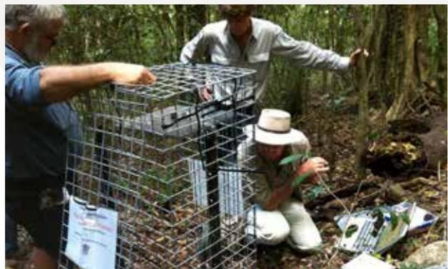
Solar powered acoustic survey equipment installed on an environmental reserve to detect endangered birds. Equipment developed by local engineers in partnership with leading acoustic software experts from a university in Japan.
