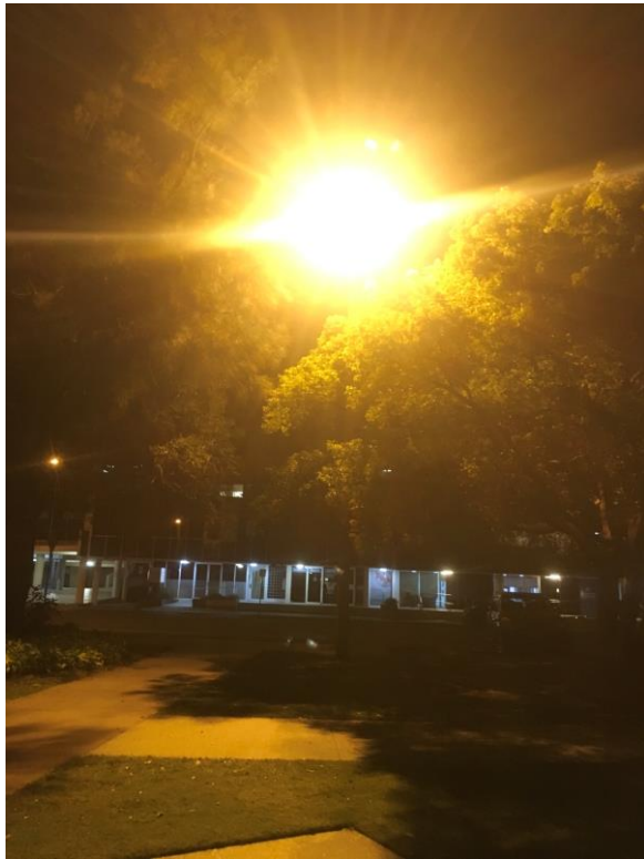
Image 24: High mounted luminaires illuminating vegetation canopies produce shadows on the ground. Vegetation is useful for screening light and reducing sky glow. Light sources mounted below the vegetation canopy will illuminate the required area using less light output and, hence, consume less energy.
