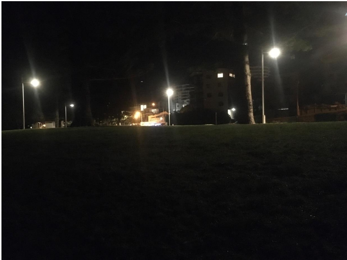
Image 30: High intensity carpark, road and footpath light sources visible from the beach due to high mounting heights and insufficient shielding.
