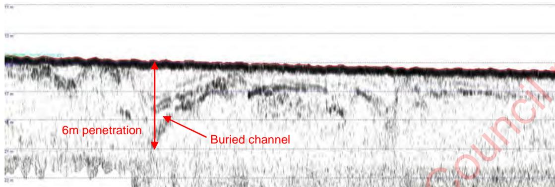
Figure 9: Example of penetration achieved with SBP. Buried channel in the northern survey block. Horizontal scale lines at 2m
