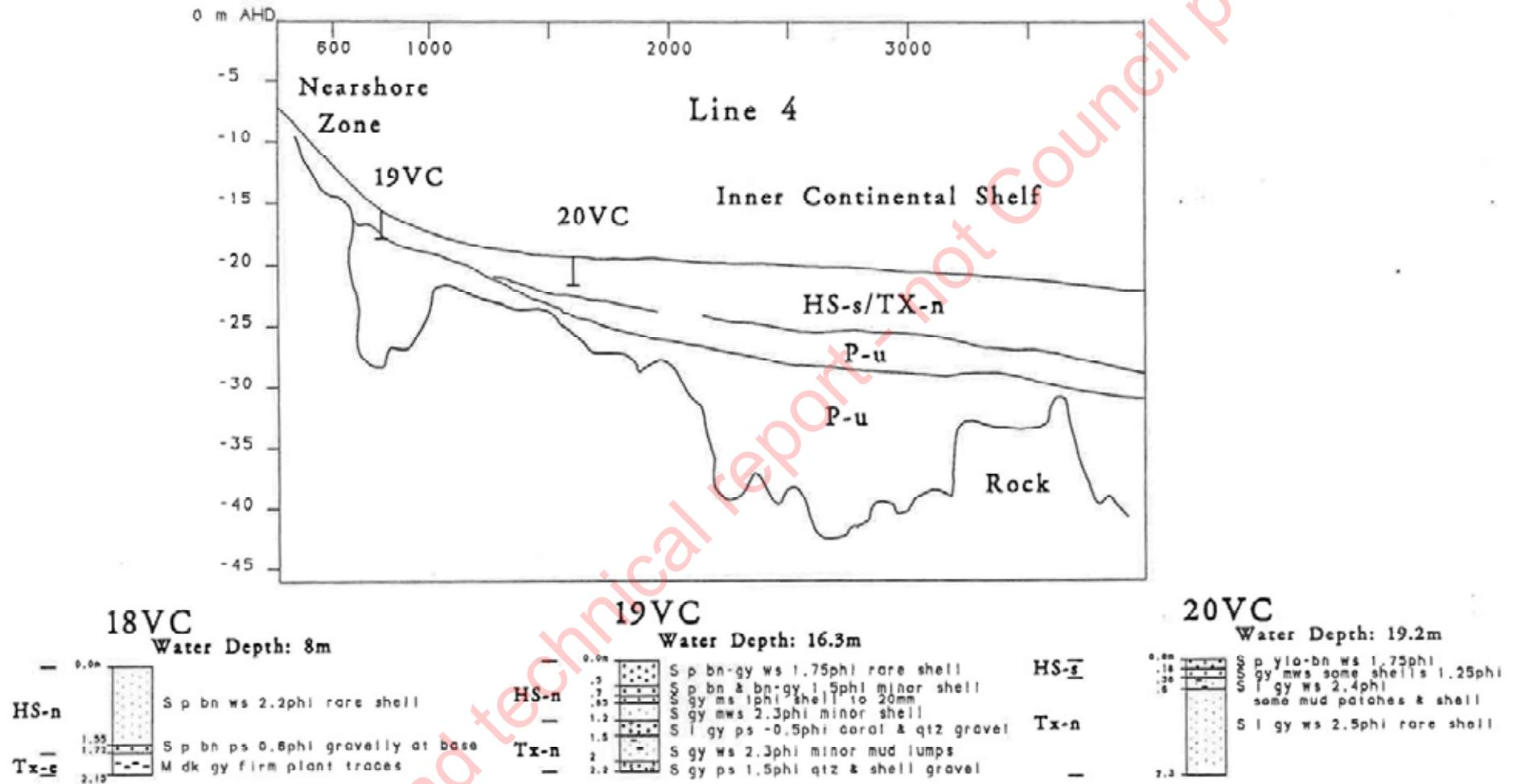
Figure 2-2 Seismic Profile and Sediment Cores East of Warana: Holocene (HS-s), Transgressional Nearshore (TX-n) and Pleistocene (P-u) Deposits (from Jones, 1992); Line 4 in Figure 2-1.
