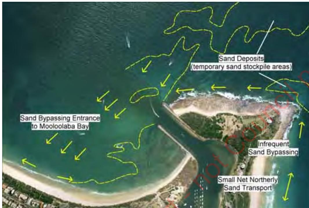
**Figure 4-3 Conceptual Model of Sand Bypassing at the Mooloolaba Harbour Entrance (modified from: Department of Harbours and Marine, 1987)**
