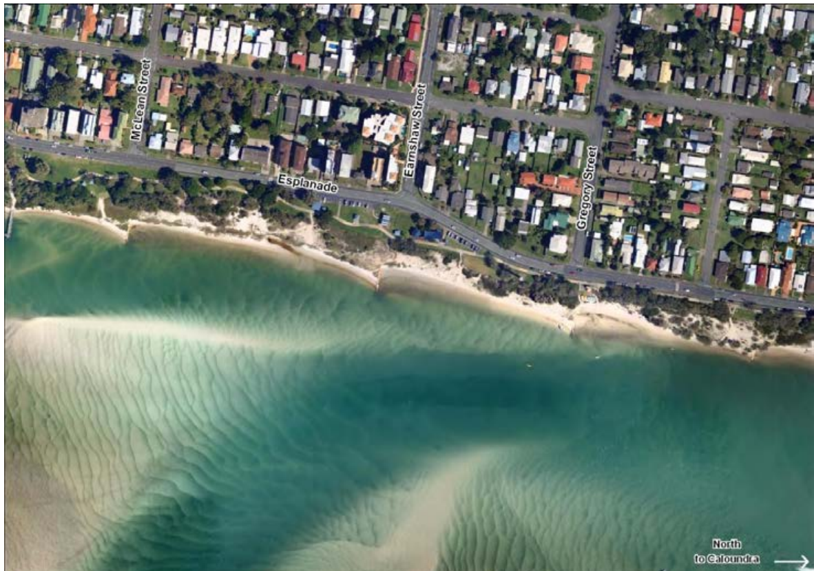
Figure 4-8 A Series of Groynes at Golden Beach (NearMap Pty Ltd, 2013)
