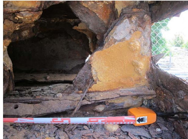
Figure 30. Close up view of one of the knees and frames inside the first hull piece. (Cosmos Archaeology, 26 September, 2014)
