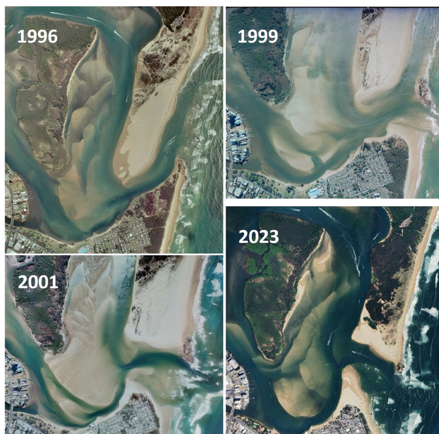
Figure 2. Changes in the configuration of the Maroochy River entrance channel 1996-2023. Contains imagery © State of Queensland 2023, © 2023 Google and © 2023 Airbus.
