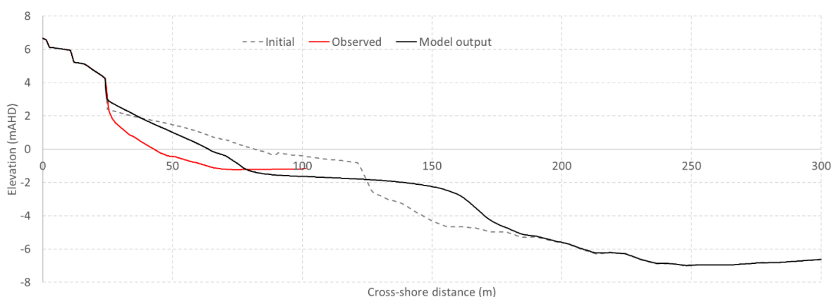
Figure 4-10: Input beach profile (dashed), output profile (black), and surveyed eroded profile (red).
