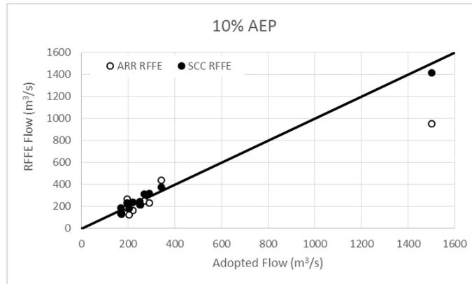
Figure 5 Comparison of SCC and ARR RFFE at 10% AEP
