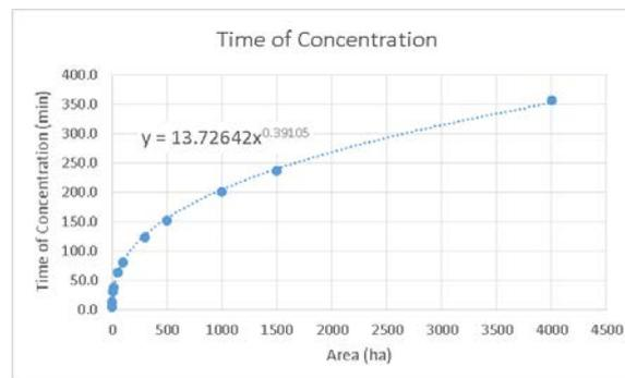
Figure 10 Time of Concentration derived from Area (CF 2.6, Slope 2.5, Imp 0%)
