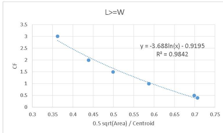
Figure 13 CF equation for catchments where Length  $\geq$  Width
