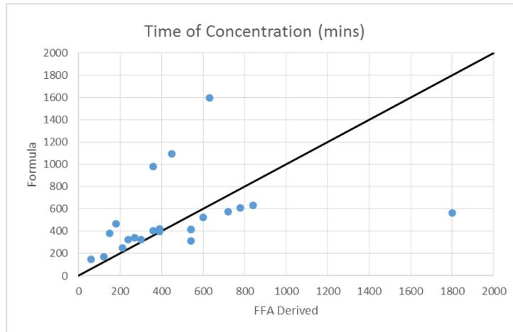
Figure 14 SCC (2017) ToC estimates compared with FFA derived ToC estimates
