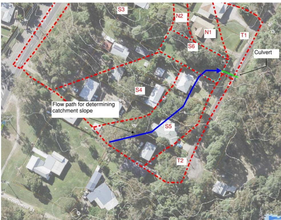
**Figure H3 – Flow Path for Determining Catchment Slope**
