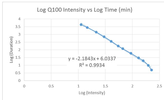
Figure 9 Log Intensity (Nambour) vs Log Duration
