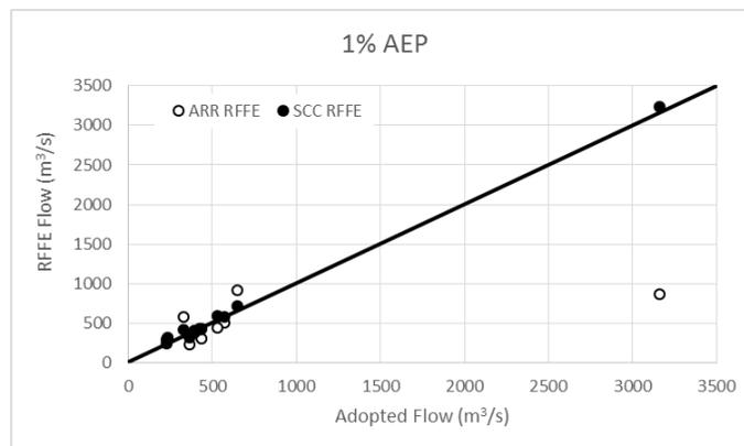
Figure 6 Comparison of SCC and ARR RFFE at 1% AEP
