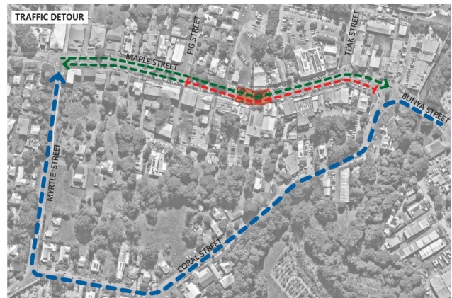
Temporary detour plan for west-bound traffic
