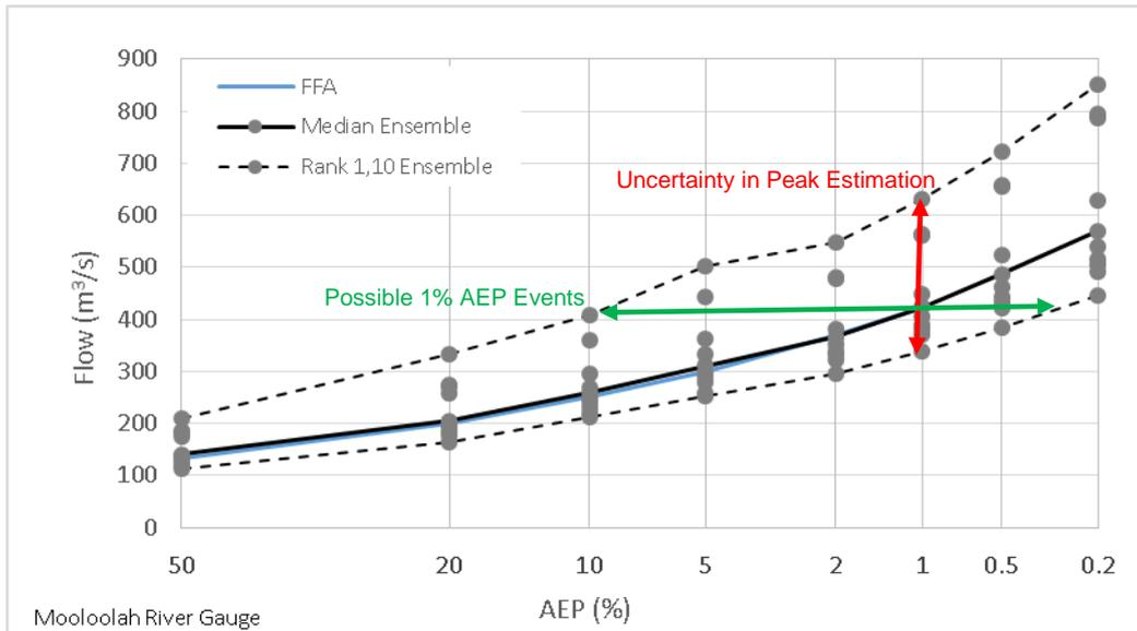
Figure 2 Comparison of the Mooloolah River FFA with Design Results derived using Ensemble Patterns
