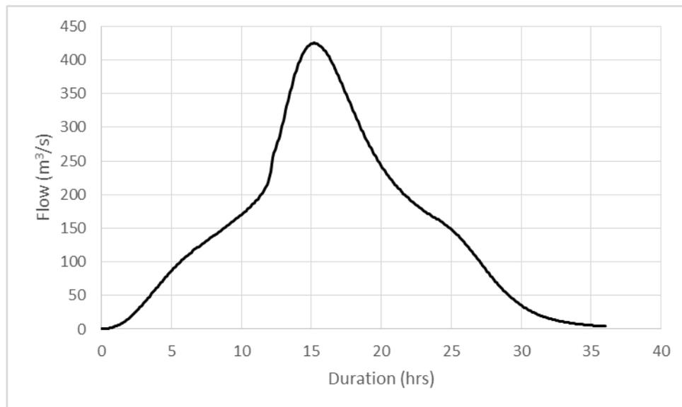
Figure 6 1% AEP Hydrograph from 24hr Duration Independent Storm Temporal Pattern
