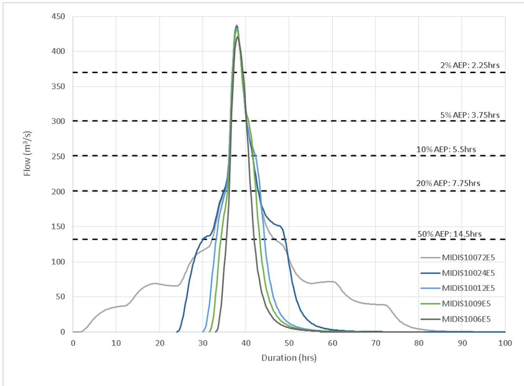
Figure 7 MIDIS 1% AEP Hydrographs for different storm durations
