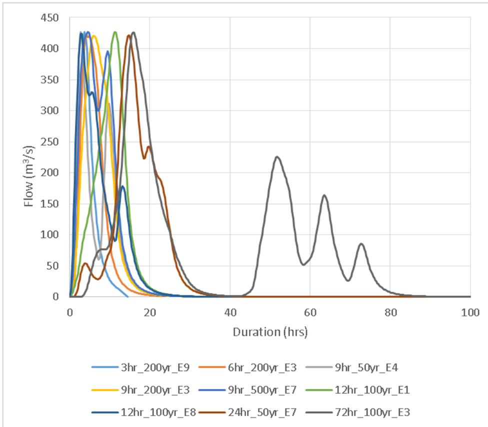
Figure 3 1% AEP Discharge Hydrographs from Ensemble Hydrographs
